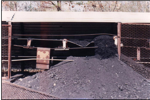
Figure 14 - Belt Spillage in progress
