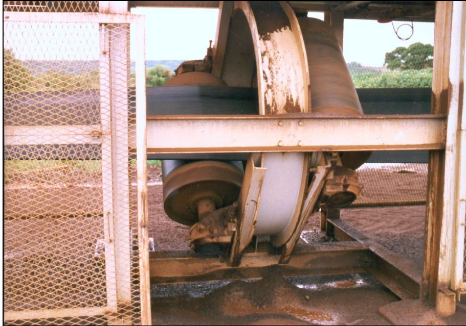
Figure 16 - Belt turnover shown at quarter point of rotation
