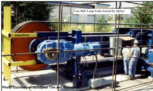
Figure 3 Splice Fatigue Test Machine
